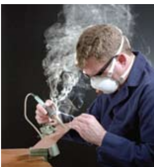
Figure 45 Soldering with and without Tyndall illumination
